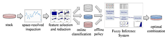
Fig. 3. Selective rotor assembly based on space-resolved inspection using feature reduction and a fuzzy inference system.
