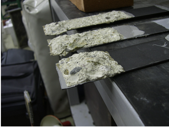
Fig. 7. Bulb at FRP anchorage, for different size and shape of the bonded area.
