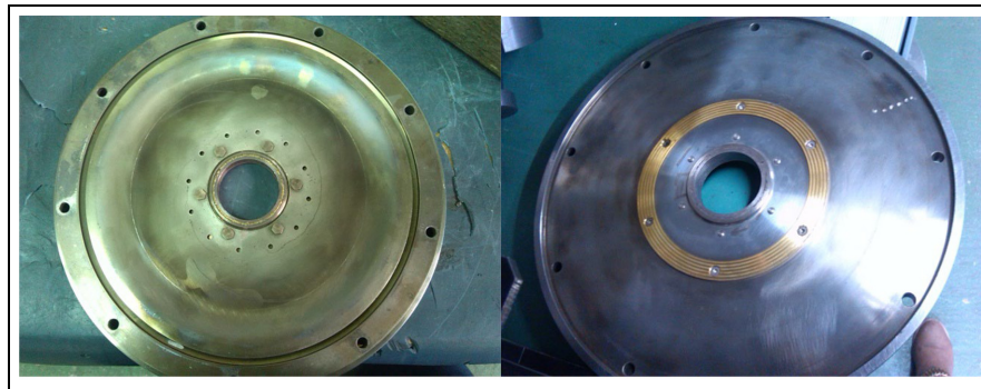
Figure 20. Multifunctional bulkhead assembly after test (side toward turbine on left and side toward compressor on right). 14
