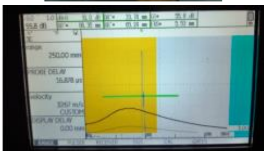
Figure 18. Ultrasonic inspection of vessel 977 - defect 1.6.
