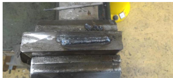
Figure 11. Welded test passes.
