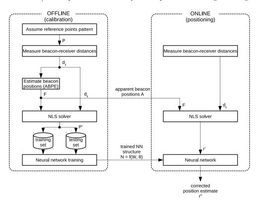
positions the beacon–receiver distances  $d_{ij}$  are measured via UWB positioning system. The distances  $d_{ij}$  and the pattern **P** are necessary as the input for the next stage of the algorithm.
