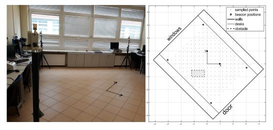
room. Four anchors were located in positions indicated in Figure 4; measurement positions were taken on every vertex of the square grid with the spacing of 0.30 m.
