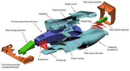
Figure 1. Exploded view of F1 vehicle
