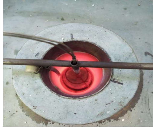
Fig. 3. The standard furnace for non-combustibility test
