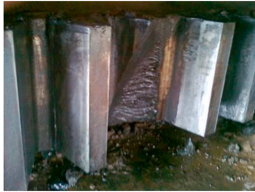
Fig. 3. Appearance of the fracture surface of the girth gear at the broken tooth spot.
