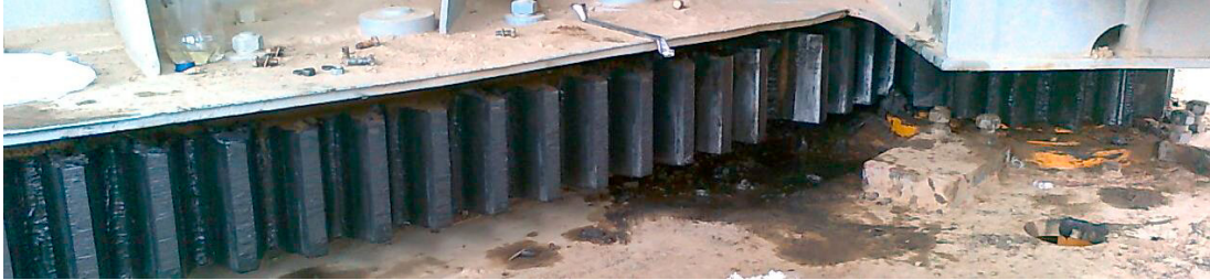
Fig. 2. Appearance of the girth gear and the pin for rotation of the excavator's upper structure.
