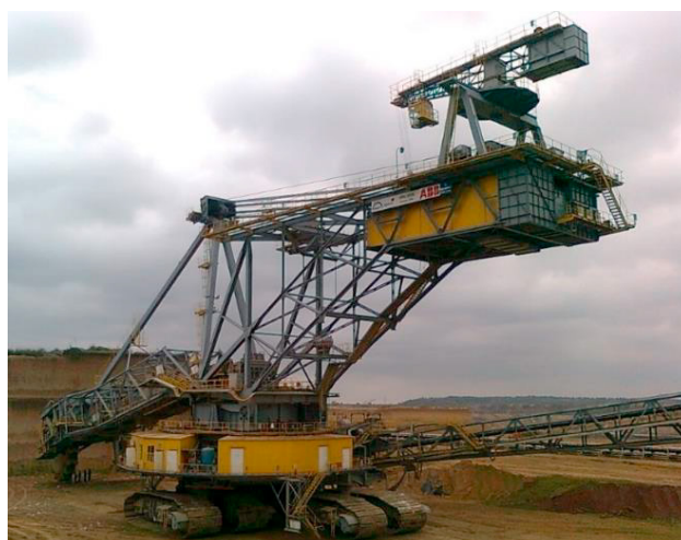
Fig. 1. Bucket wheel excavators SRs 2000 x 32/5.0 "Kostolac" (Serbia).
