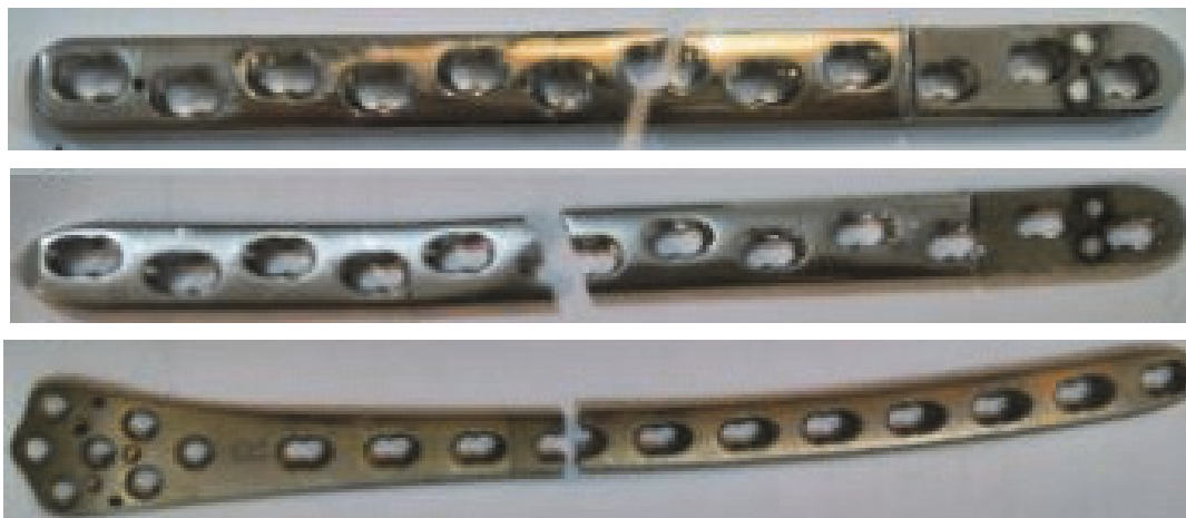
Figure 1. Typical failures of LCP caused by fatigue, [1],
