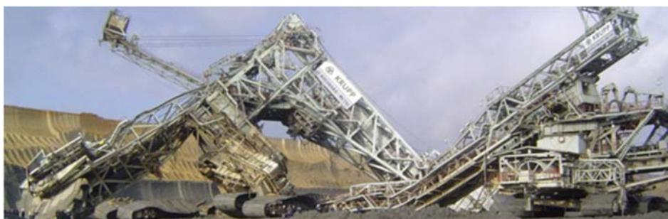
Fig. 1. Collapse of bucket wheel excavator SRs 1760.
