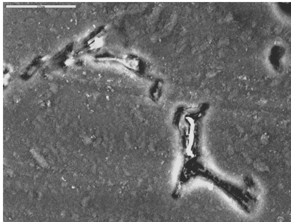
Figure 3 Porosity of sample with the shortest degasification time
