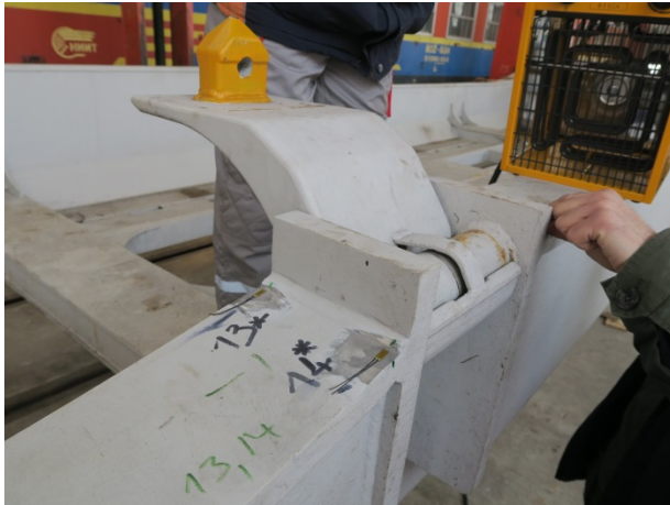
Figure 5. Applying the strain gauges on the testing object.
