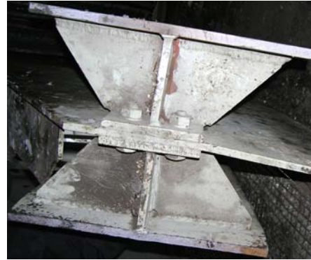
Figure 18. View of fractured assembly: combined fracture of right lug and brittle fracture of lug, left in Fig. 17 (lower part). Slika 18. Izgled loma sklopa: kombinovani lom desne uške i krti lom uške, levo na sl. 17 (dole)
