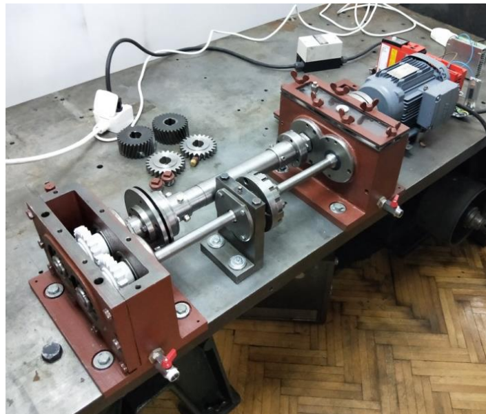
Fig. 2 Back to back gear test rig used in performed experimental research
