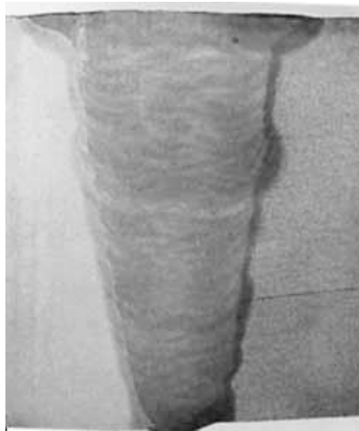
Figure 3. Welded joint macro recording
