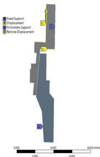
Figure 3. 2D FE model with symmetrical BCs and applied displacement
