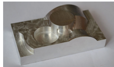
Fig. 5. The test piece used in case study 1 – machined part with planar surfaces parallel to coordinate axes.
