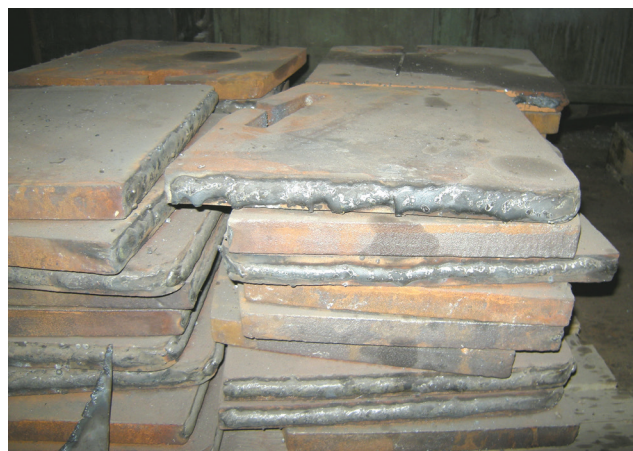
Figure 7. Hardfaced suction plates.
