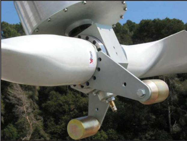
Figure 8: Built-composite blades W55RBVS
