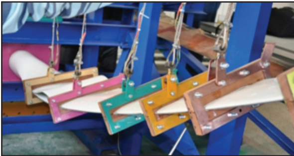
Figure 16: The position of the blade fracture
