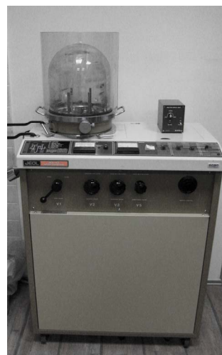
Figure 2. Vacuum deposition technique (NanoLab 1, Faculty of Mechanical Engineering, University of Belgrade)
