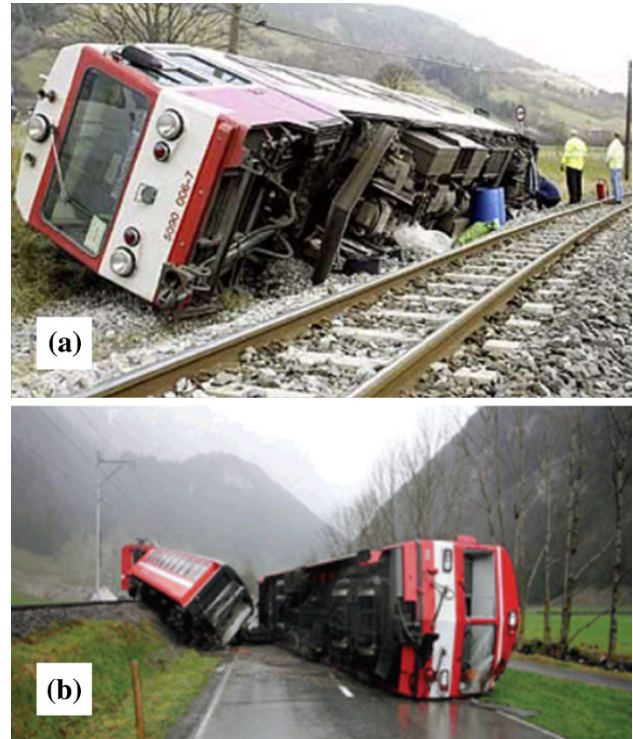
Fig. 2 Crosswind related accidents in Austria in 2002 (a) and Switzerland in 2007 (b) [3, 4]
