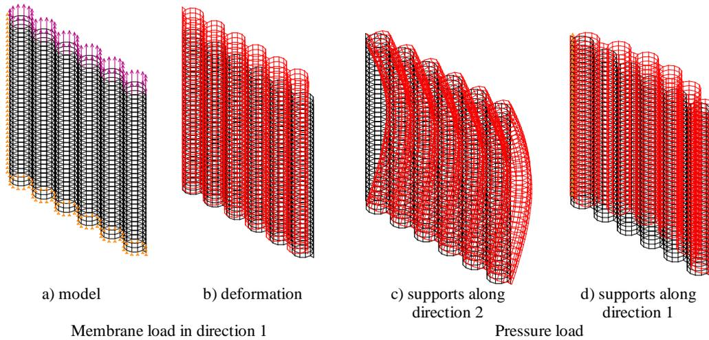
**Figure 1. Membrane wall under the load in direction 1 and under the pressure load**
