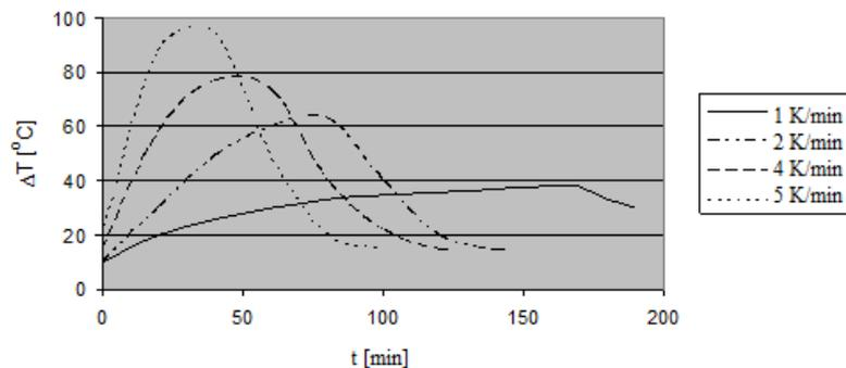
**Figure 10. Temperature differences between membrane wall and internal buckstay as a function of time and heated velocities**
