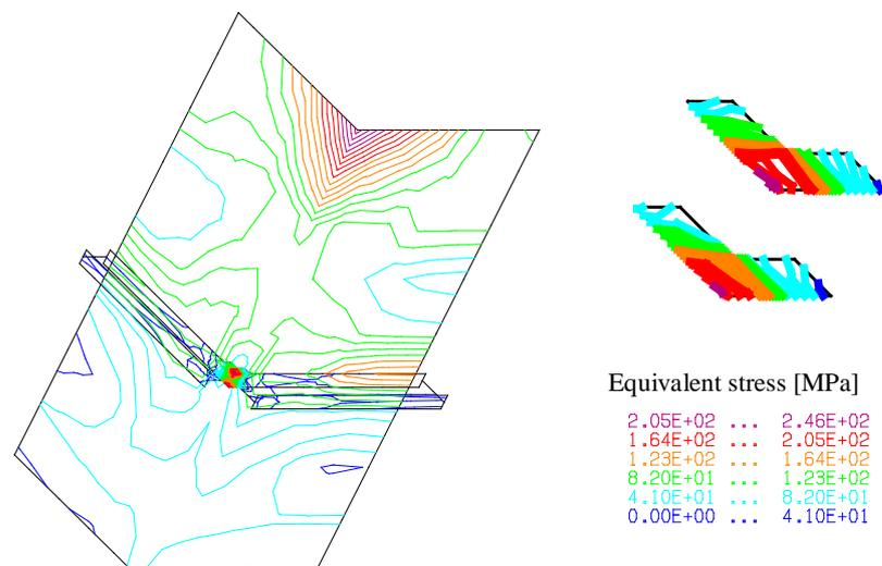
**Figure 13. Deformation and stress calculated from model M3**
