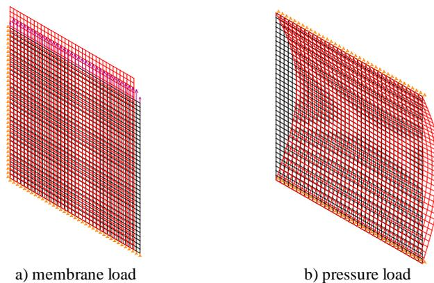
**Figure 2. Deformation of the plate**
