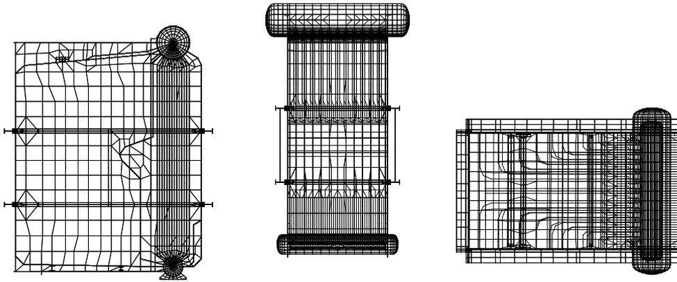
Figure 5. FEM model of the boiler construction
