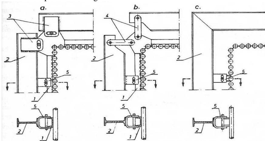
1. Internal buckstay 2. External buckstay 3. Connecting slider of external buckstays
