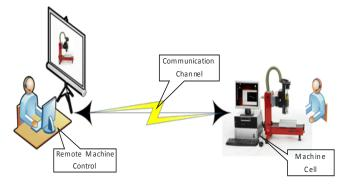
Figure 1. Human – Machine Communication channel for remote control
