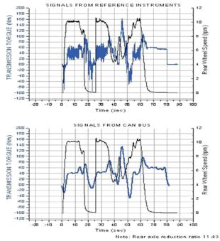
Figure 12 Comparison between data provided through reference instruments (top) and CAN bus (bottom) for transmission torque and rear wheel rpm. Conditions: Bare tractor, acceleration and deceleration.
