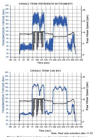
Figure 11 Comparison between data provided through reference instruments (top) and CAN bus (bottom) for transmission torque and rear wheel rpm. Conditions: bare tractor, constant speed.
