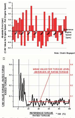
Figure 10 Analyses of the difference between CAN value for engine speed and reference engine speed (top) and CAN value torque and reference torque (bottom)
