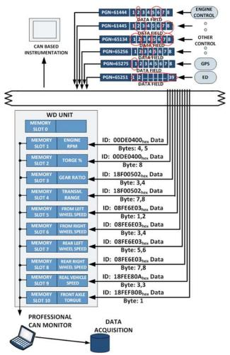
Figure 8 Concept of the measurement
