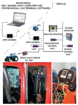
Figure 7 System for service load data acquisition trough CAN bus: top – configuration of the system, bottom left – EM built in the tractor; bottom middle – GPRS modem built in the tractor, bottom left – installation of the WD unit
