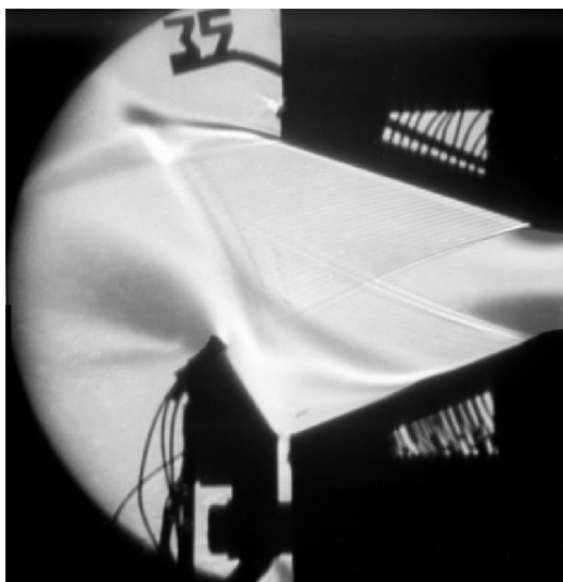
Figure 5. Data from measurements: Schlieren photo and initial separation point characteristics
