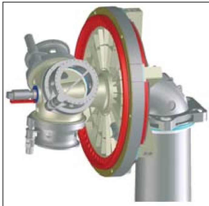
Figure 2. Direct drive of Enercon E-48 [17]
