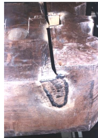
Figure 8. Appearance of the ram after the hard facing
