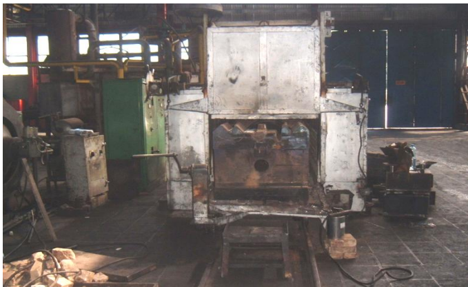
Figure 7. Preheating of the ram in the horizontal electroresistance furnace
