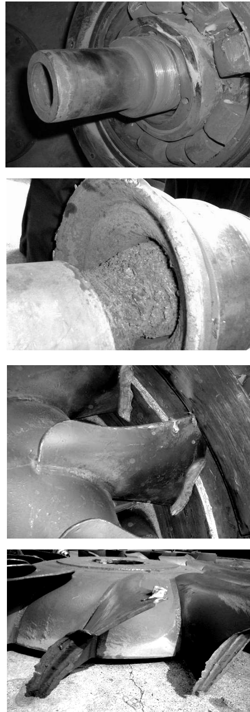
Figure 2. Different types of damages of rotating system components.
