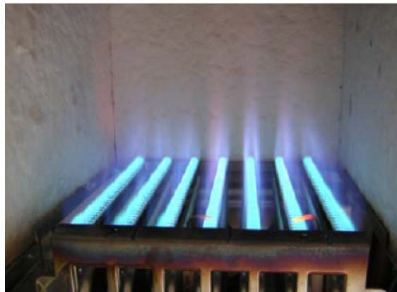
Figure 17. Combustion chamber and burner
