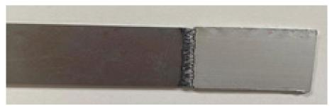
*Fig.2.* Sample of aluminum and iron welding
