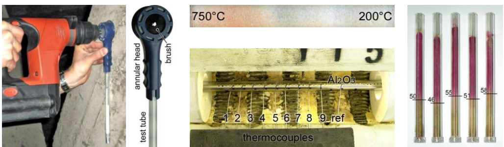
Figure 4. The Carbontest ® tool for collecting the drilling powder, discoloration of a powder sample, setup for the multiple Differential Thermal Analysis, de-alkalinization depth in the panel of Fig. 3 (scale 2:1, in mm).
