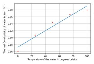
Figure 2: A plot of water's thermal conductivity against its temperature
