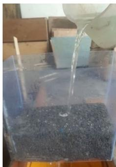
Gambar 3. Uji Permeabilitas *Porous Paving Block*
