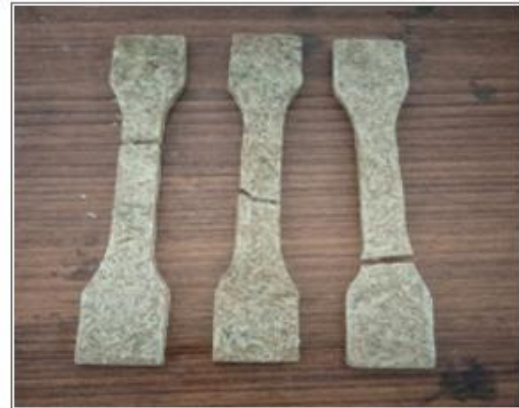
Gambar 4. Hasil uji Tarik 80% resin, 20% komposit
