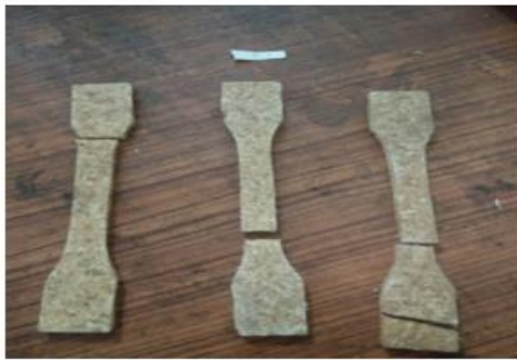
Gambar 6. Hasil uji Tarik 90% resin, 10% composite
