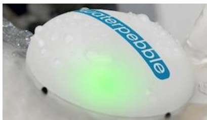
Figure.3 Water pebble gives real-time feedback about the water consumed during a shower. It changes its color from green to red to communicate to the user that the consumption is getting unsustainable.
