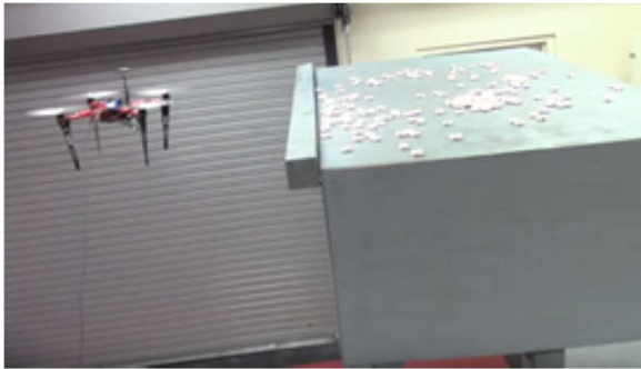
Figure 17: Hosing top of bridge deck
