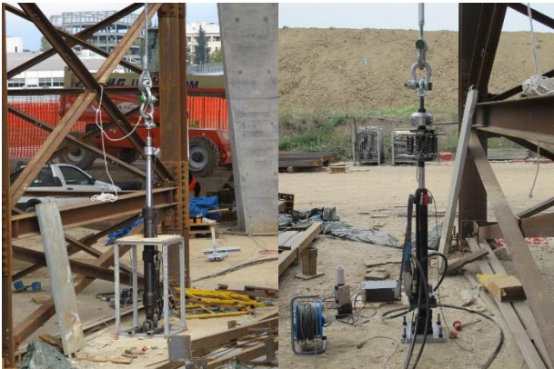
Figure 5. (sx) impulsive excitation (dx) harmonic excitation
