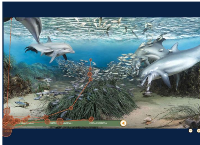
Figure 3. Scanpath of a subject during the execution of task 1. Circles represent fixations, straight lines saccades
