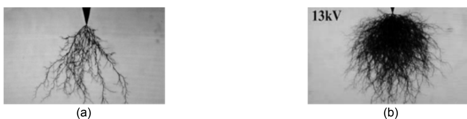
Figure 2: Electrical tree structures in a XLPE cable insulator. In (a) a branch-like structure while in (b) a bush-like structure (Xiangrong et al., 2011)
