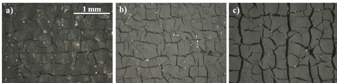
Figure 2. Optical microscope images of MPL surfaces: (a) GDM-PTFE; (b) GDM-PFPE-12; (c) GDM-PFPE-6 (40×).
