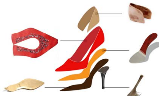
Figure 1: Flexible and structural components of a shoe.
