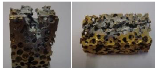
Fig. 1. Trial of joining of the foam in the bead on plate configuration
