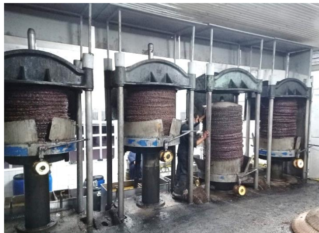
Figure 8. Pressing by the Traditional System with the use of pressing mats.
