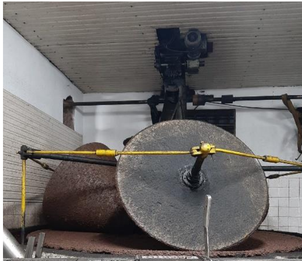
Figure 6. Stone crushing milling structure.
