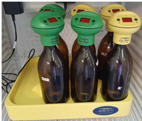
Figure 33. OxiTop bottles used in the BOD 5 analysis.
