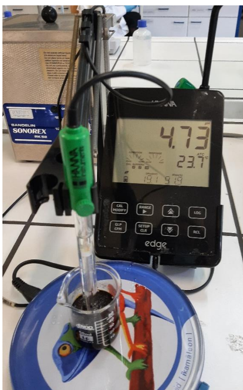
Figure 27. HANNA multiparameter meter used for the pH and electric conductivity analysis.
