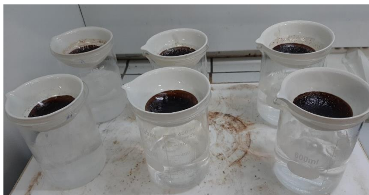
Figure 31. Apparatus for the evaporation step of Total Solids.
