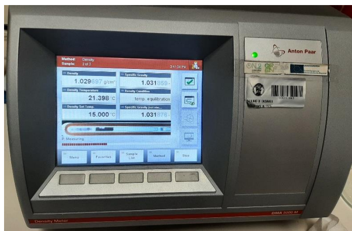
Figure 26. Anton Paar densimeter used in the density analysis.
