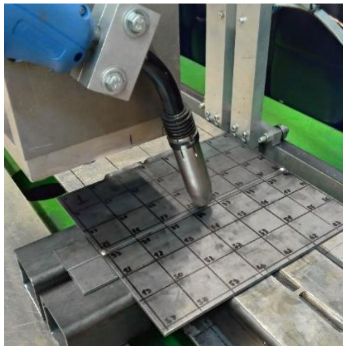
Figure 8. Arrangement without movement restrictions during the welding process in top joints.
