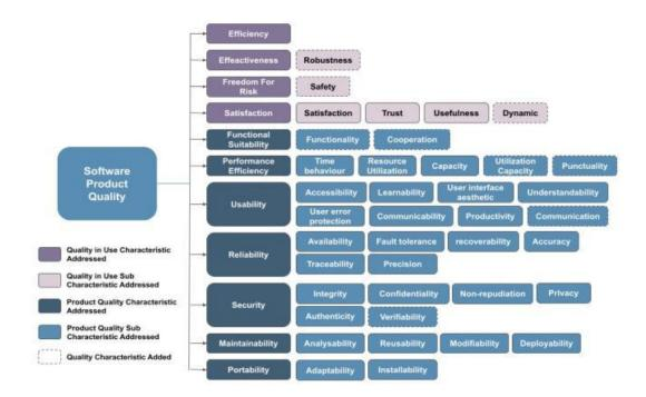
Figure 2: Overview of the NFR grouping analysis from ISO/IEC 25010.
