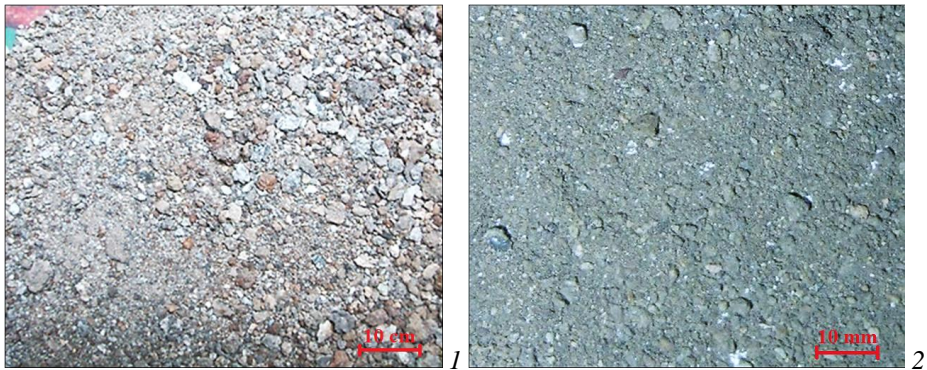
Fig. 2. Aluminum-bearing slag before sorting and mechanical separation (extraction) of metal inclusions, with a particle size of 1-50 mm (1) and after, - particles with a size of 0-5 mm (2).
