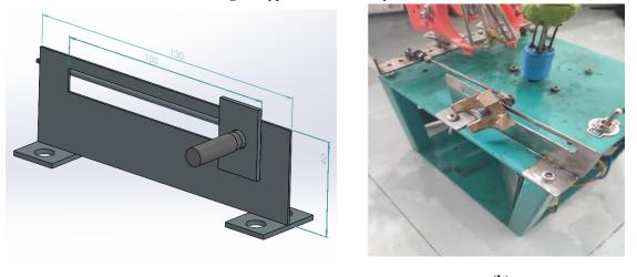
(a) (b) Fig.5. The slider and the push and pull mechanism. (a) CAD model, (b) Real production.
