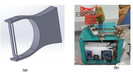
Fig.6. The cutting tool. (a) CAD model, (b) Cutting tools locating on the machine.
