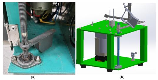
Fig.9. The spindle and lead screw nut.
