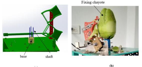
(a) **Fig.3.** Rotating shaft with chayote fixing. (a) CAD model; (b) manufactured chayote peeling machine.
