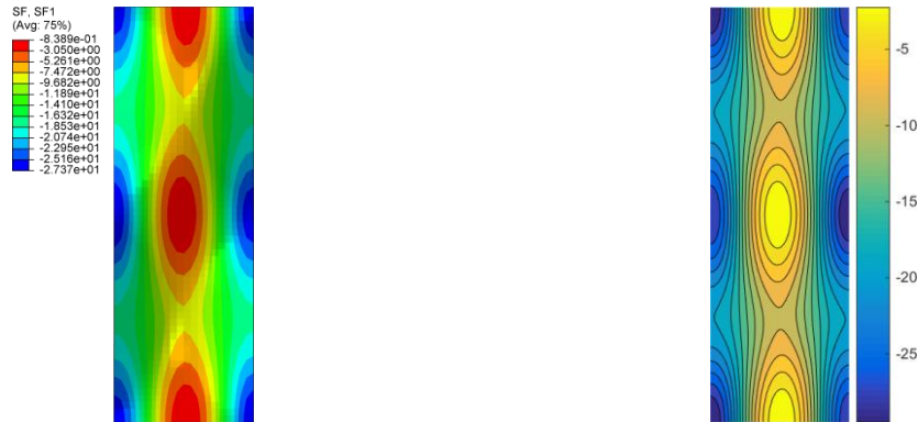
Figure 3: Contour of N_{xx} for Panel 2 at P/P_{buck} = 3.0 : (a) analytical, (b) Abaqus.
