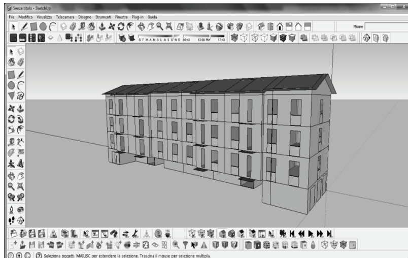
Fig. 2. Geometrical model for Trnsys by means of Google SketchUp.
