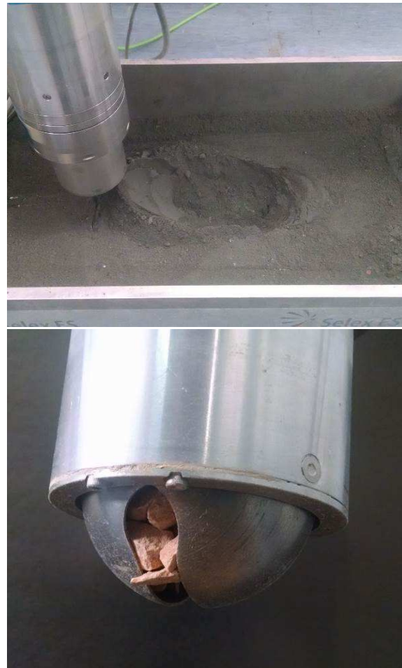
Figure 8-1: Some images taken during the test campaign with M soil (top) and G soil (bottom)
